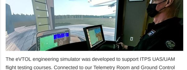
Station (GCS) with real-time data monitoring by engineers, it allows the rehearsal of piloted, remotely piloted, and autonomous eVTOL flight test operations. The eVTOL simulator cockpit allows for multiple control configurations to evaluate different Human Machine Interface (HMI) strategies. Piloted evaluations feature a mixed reality solution providing a high degree of realism. The design is based on a Bell 206 to represent a machine with potential UAM or utility applications.
