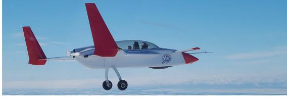
The Adaptive Handling Qualities Aircraft (AHQA) has completed Phase 1 testing and is now conducting Phase 2 aimed at establishing the in-flight demonstration exercises. AHQA will be employed in support of our Flying Qualities and Digital Flight Control Systems (DFCS) courses. This unique aircraft provides students a real-time testing of handling qualities while linking to the Telemetry Room for a team training experience.
